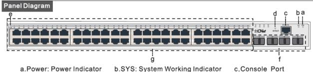
a.Power: Power Indicator b.SYS: System Working Indicator c.Console Port d.Default e.L/A: Port Link/activity Indicator f.Uplink Port-1X~4X Port: 10G SFP+ g.PoE Port -1~48 Port: 10/100/1000M RJ45 Port(PoE Ports)
